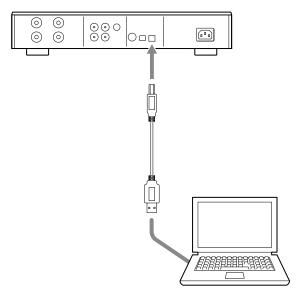
The cable must match the connection terminal of this unit (USB-B type).
